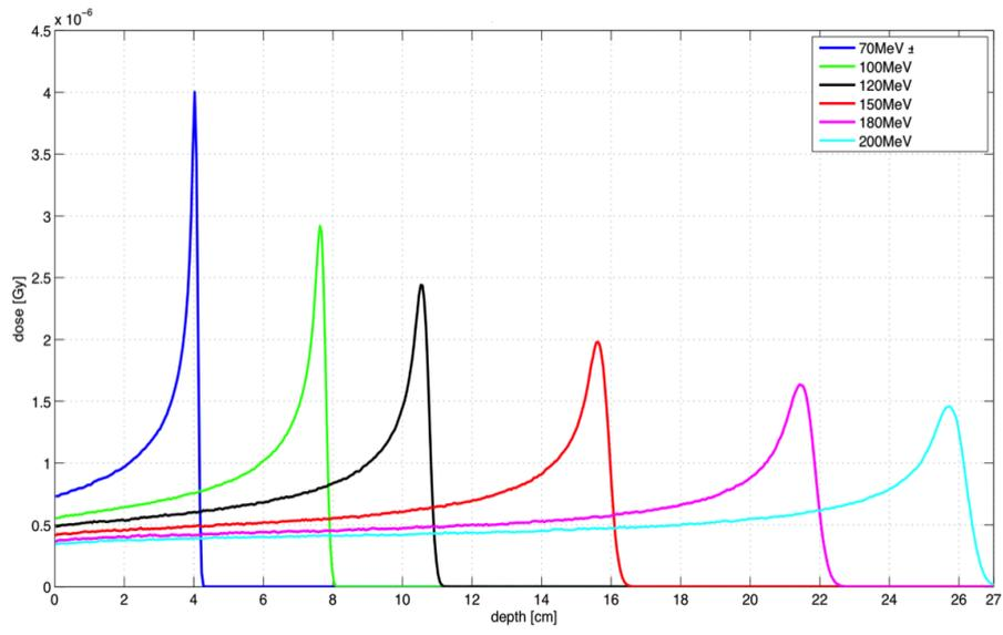
**Fig. 2.** Example of 'pristine' Bragg peaks based on Monte Carlo calculations to be used as input data for beam modelling and dose calculation
